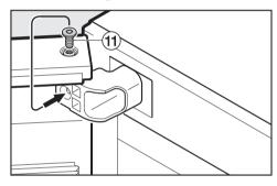
Remove screw ① from the hinge pin and screw it into the drill hole in the bearing block.
